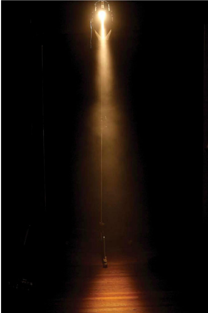
The light from this 300W Fresnel can be seen in a beam projecting out from the fixture because it is backlighting the fog in the air. Keeping it against a black background helps to accentuate the light beam.
